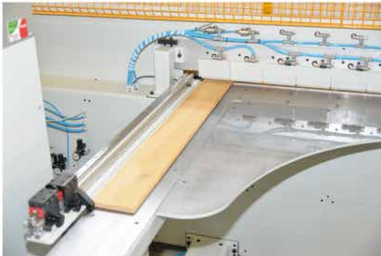
VERSION FOR THE ENDPROFILING OF TILES. Max width 220 (optional 400 mm). Random lenght unlimited.
