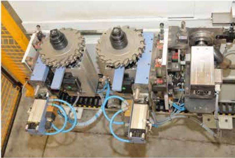
CARRIAGE GROUP FOR SUPPORTING THE WORKING MOTORS IN DIFFERENT VERSIONS (see drawings)
